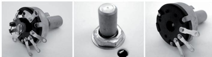
Volume control with switch and feedback controller (Potentiometers)
